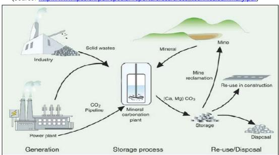
**Figure 9.** Process of converting gaseous CO<sub>2</sub> into stable solid mineral carbonates. (Source: <u>http://www.ipcc.ch/pdf/special-reports/srccs/srccs\_technicalsummary.pdf</u>)
