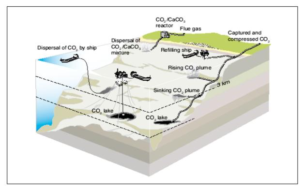
Figure 8. Various methods proposed for storing CO<sub>2</sub> in the oceans.
